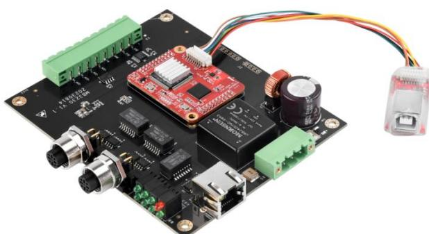
When DMS-UART-8P configuration cable is connected to the management computer USB interface, the computer will add a USB simulation serial port.
