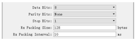
When converting the byte stream of UART into UDP message or HDLC frame, if every byte is converted into a UDP message for transmission, the overhead is too large and the efficiency is too low.
