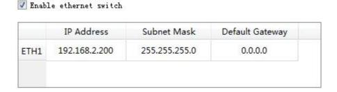
After enabling the Ethernet switching function, HDLC-ATC only has one IP address. The network functions are as follows:
