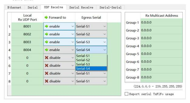
The following configuration implements an application that receives data from a UDP port and distributes it to eight serial ports simultaneously:
