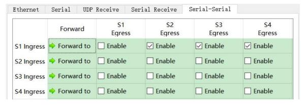
As shown in the above figure, the input of serial port S1 is split to the output of S2, S3 and S4. HDLC-LCM stores and forwards the receiver, even if the baud rate and clock mode of S1, S2, S3 and S4 are different, it will not lose packets.
