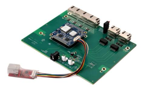
When DMS-UART-8P configuration cable is connected to the management computer USB interface, the computer will add a USB simulation serial port.
