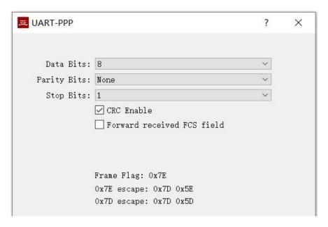
The UART-PPP frame format adds 0x7E before and after the packet as the opening flag closing flag with the frame structure as follows:
