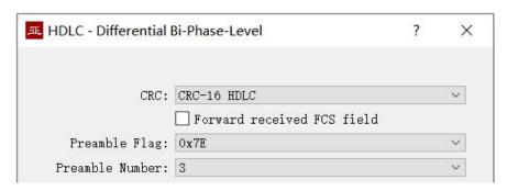
It is important to note that many claims that DBPL encoding is in fact differential Manchester encoding, so users need to carefully refer to the definition of the Synchronous Serial Encoding Format chapter to choose the correct working mode.
