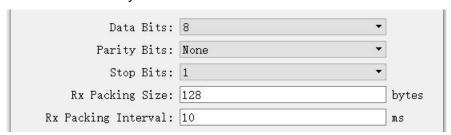
When converting the byte stream of UART into UDP message or HDLC frame, if every byte is converted into a UDP message for transmission, the overhead is too large and the efficiency is too low.
