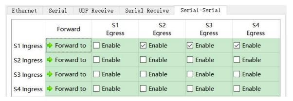
As shown in the above figure, the input of serial port S1 is split to the output of S2, S3 and S4. HDLC-ATC stores and forwards the receiver, even if the baud rate and clock mode of S1, S2, S3 and S4 are different, it will not lose packets.
