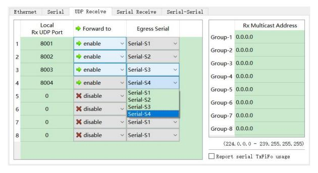
The following configuration implements an application that receives data from a UDP port and distributes it to four serial ports simultaneously:
