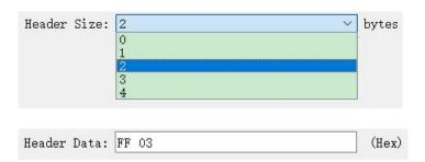
The above figure is taken as an example. The length of frame header is defined as 2, and the content of frame header is defined as FF 03 in hexadecimal:
