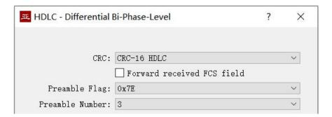
It is important to note that many claims that DBPL encoding is in fact differential Manchester encoding, so users need to carefully refer to the definition of the Synchronous Serial Encoding Format chapter to choose the correct working mode.
