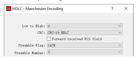
In addition to the same configuration parameters as NRZI, the Manchester encoding format has parameters with the meaning of edges with low to high waveforms for data lines:
