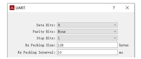
When converting the byte stream of UART into UDP message or HDLC frame, if every byte is converted into a UDP message for transmission, the overhead is too large and the efficiency is too low.
