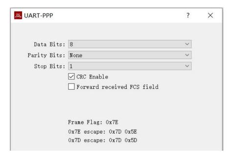
The UART-PPP frame format adds 0x7E before and after the packet as the opening flag closing flag with the frame structure as follows:
