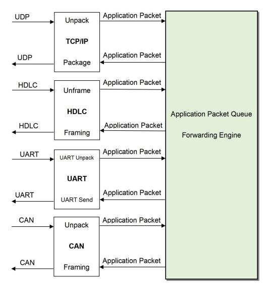
At the time of receiving, the receiving processing modules of different types of interfaces perform unpacking or decoding operations on the data, extract the application data packets, and send them to the queue of the system.
