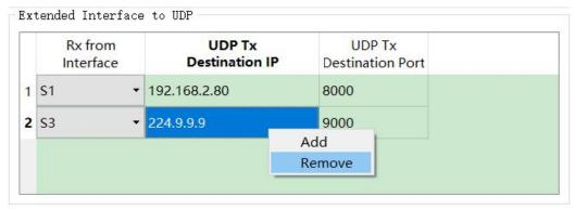
According to the application requirements, "UDP Tx Destination IP" can be unicast, multicast or broadcast address.
