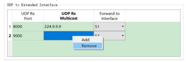
If you want to receive multicast messages, you must fill in a valid multicast address in the 'UDP receive multicast address' table. If only unicast or broadcast messages are received, the form will not be filled in or filled in with 0.
