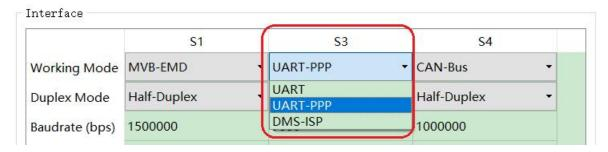
After determining the working mode, the contents of the "Advanced Options" cell will be adjusted automatically according to the working mode.
