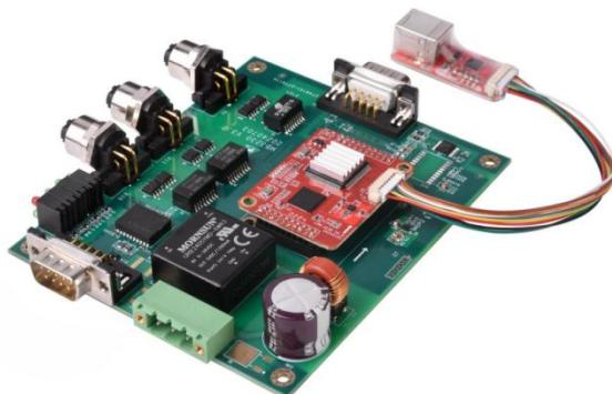
When DMS-UART-8P configuration cable is connected to the management computer USB interface, the computer will add a USB simulation serial port.
